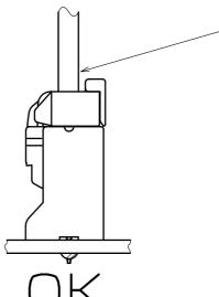
No stress concentration: No cable bending close to connector
