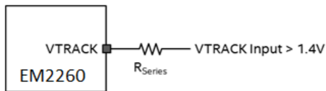
Figure 13: VTRACK Sense Circuitry (Input > 1.4V)
