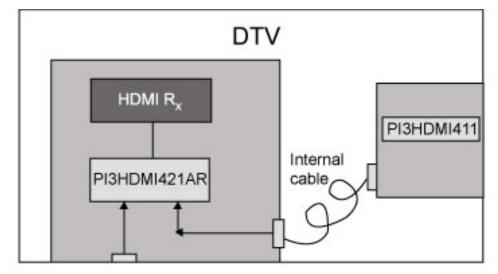
Figure 1: DTV with 2 HDMI<sup>™</sup> connectors (1 HDMI<sup>™</sup> in back & HDMI<sup>™</sup> on the side)
