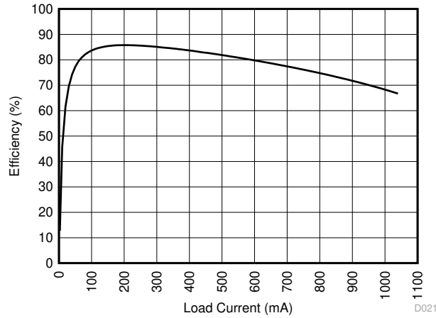
SN6505B + Würth 750316028 V_{CC} = 3.3\text{ V}
