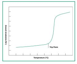
Understanding the differences in performance between the two types of devices will make the best circuit protection choice easier. The most obvious difference is that the PTC is resettable. This is an inherent characteristic in which the PTC resets (returns to low resistance state) after power is removed and the device cools down. There are a number of other operating characteristics that differentiate the two types of products.
