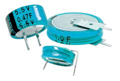
Type EDC, 70 °C electric double layer supercapacitors offer high capacitance values in a thru hole stacked coin type package. Primarily designed for integrated circuit voltage backup, the capacitors can also be used to deliver the initial power from batteries.
