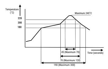
Note: Temperature profile shows printed circuit board surface temperature on the relay terminal portion. Please consult KEMET if you wish to use a temperature profile other than above.
