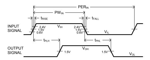
Figure 3: Timing Diagram
