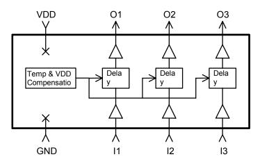
Figure 1: 3D7323 Functional Diagram
