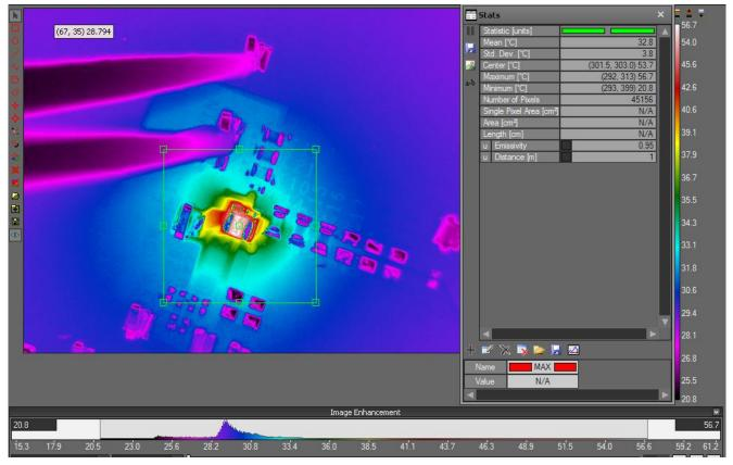
Figure 28 Thermal image at PV<sub>IN</sub> = 12V, V<sub>OUT</sub> = 3.3V, I<sub>o</sub> = 4A, room temperature, no airflow, FS1404 maximum temperature = 57°C
