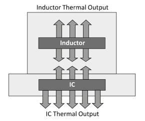
Figure 29 Heat sources in the FS1404
