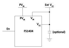
Figure 7 Using an external bias voltage
