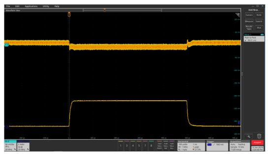
Figure 27 Transient response 0A to 4A (Ch6:I<sub>o</sub>, Ch2: V<sub>out</sub>), peak-peak deviation=40mV
