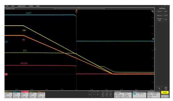
Figure 19 Shutdown with Enable de-assertion at 4A load (Ch1:PV<sub>IN</sub>, Ch2: V<sub>OUT</sub>, Ch3: PGood, Ch4:V<sub>CC</sub>, Ch5: Enable)
