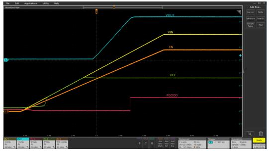
Figure 17 Startup with no load (Ch1:PV<sub>IN</sub>, Ch2: V<sub>OUT</sub>, Ch3: PGood, Ch4:V<sub>CC</sub>, Ch5: Enable)
