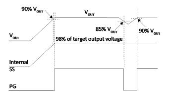
Figure 15 PG signal when PGControl bit=0
