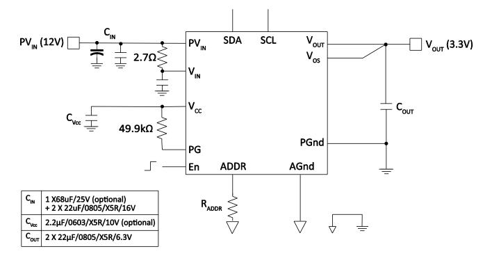
Figure 16 Application circuit for a single supply, PV<sub>IN</sub>=12V, V<sub>OUT</sub>=3.3V, 4A
