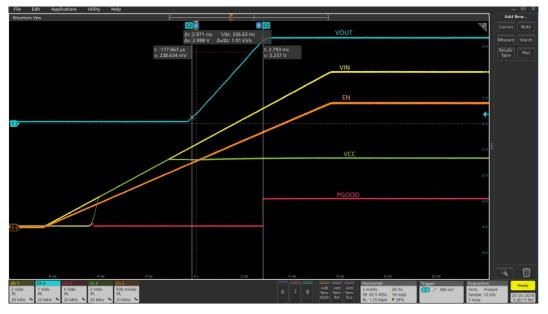
Figure 18 Startup with 4A load (Ch1:PV<sub>IN</sub>, Ch2: V<sub>OUT</sub>, Ch3: PGood, Ch4:V<sub>CC</sub>, Ch5: Enable)
