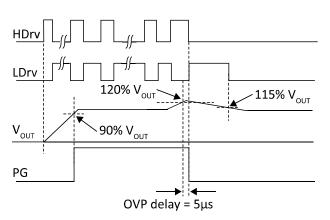
Figure 13 Illustration of latched OVP
