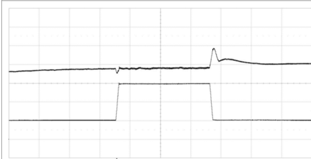
Output voltage response to load current Top trace: output voltage (100 mV/div.). Step-change (10-30-10 A) at: Bottom trace: load current (10 A/div.). T_{P1} = +25^\circ C , V_I = 12 V , V_O = 1.0 V Time scale: (0.1 ms/div.). di/dt = 2 A/\mu s , f_{sw} = 320 kHz C_O = 4000 \mu F
