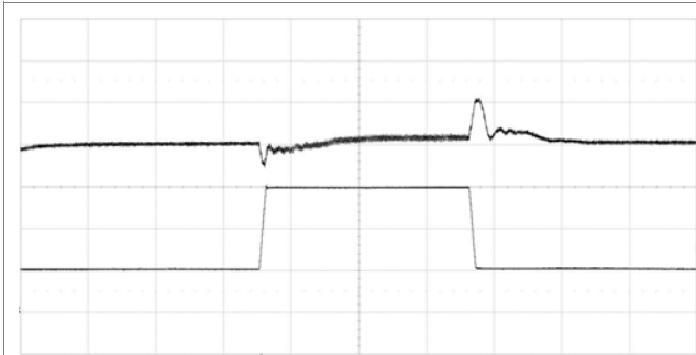
Output voltage response to load current Top trace: output voltage (200 mV/div.). Step-change (10-30-10 A) at: Bottom trace: load current (10 A/div.). T_{P1} = +25^\circ C , V_I = 12 V , V_O = 1.0 V Time scale: (0.1 ms/div.). di/dt = 2 A/\mu s , f_{sw} = 320 kHz C_O = 4000 \mu F
