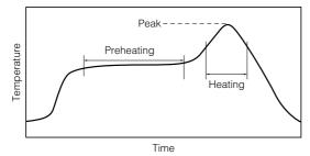
Recommended soldering conditions for flow
