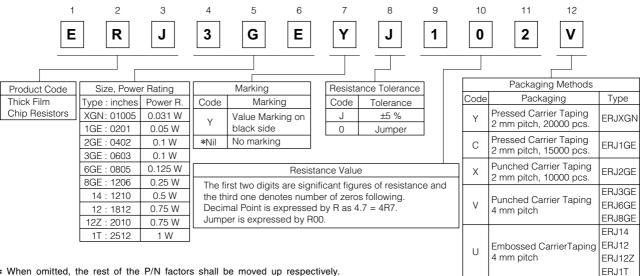
\* When omitted, the rest of the P/N factors shall be moved up respectively. (Only XGN, 1GN, 2GE type)
