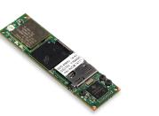
Get the best of wireless communications, graphics processing and extended-temperature components with the Overo® IronSTORM-BY computer-on-module. With a DaVinci Digital Video Processor for graphics and featuring access point mode, 802.11b/g/n WiFi and Bluetooth 4.1 with BLE using TI's WiLink 8 wireless module, the Overo® IronSTORM-BY COM has all the features you need for your wireless graphics project.
