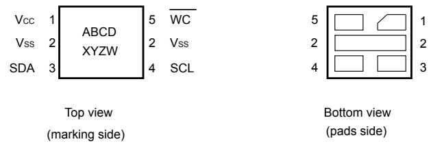
Figure 3. UFDFPN5 (DFN5) package connections
