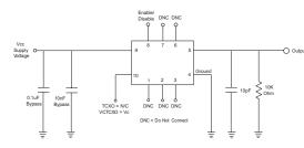
TV Series Clipped Sinewave Test Circuit
