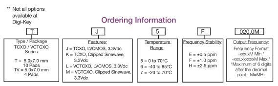
Example 1: TJ5F-020.0M = 5x7mm, TCXO, LVCMOS, 3.3Vdc, 0 to 70°C, ±1.0ppm, Output Frequency 20.0MHz
