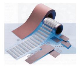
Sil-Pad 400 is a composite of silicone rubber and fiberglass. It is flame retardant and is specially formulated for use as a thermally conductive insulator. Primary use is to electrically isolate power sources from heat sinks.
