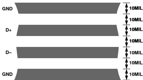
Figure 18. Arrangement of Signal Tracks
