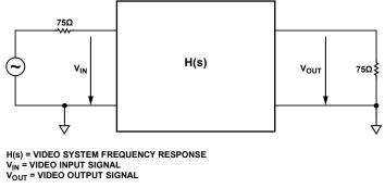
Figure 1. Video System Frequency Response
