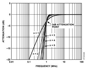
Figure 5. High-Pass Butterworth Frequency Response
