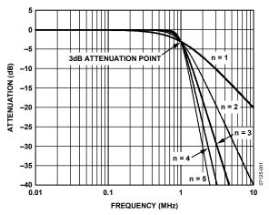
Figure 2. Low-Pass Butterworth Frequency Response
