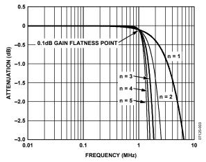
Figure 4. Low-Pass Cutoff Frequencies for Normalized Systems (0.1 dB Flatness)
