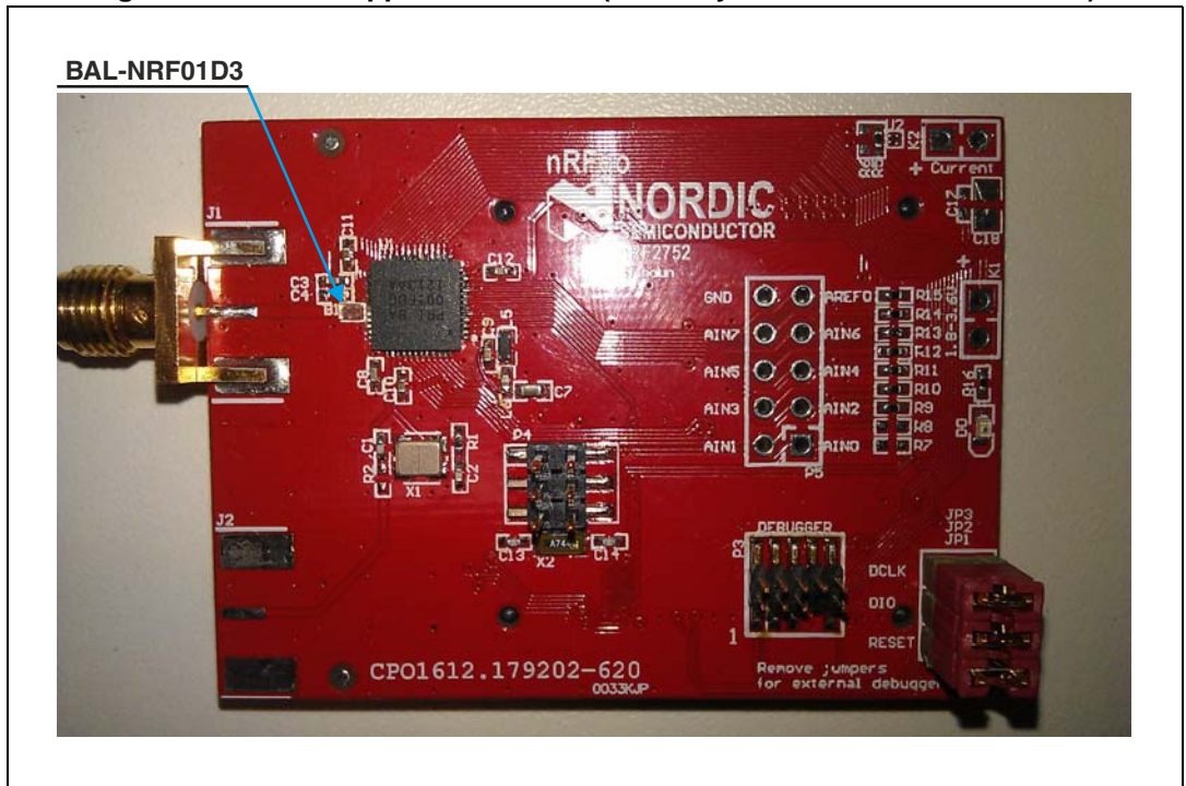
Figure 9. nRF2752 application board (courtesy of Nordic Semiconductor)
