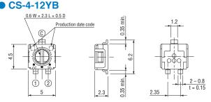
Unless otherwise specified, tolerance: ± 0.3 (Unit: mm)
