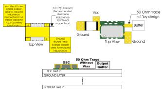
Attention: To achieve optimal frequency stability, and in some cases to meet the specification stated on this data sheet, it is required that the circuit connected to this TCXO output must have the equivalent input capacitance that is specified by the nominal load capacitance. Deviations from the nominal load capacitance will have a graduated effect on the stability of approximately 20 ppb per pF load difference.
