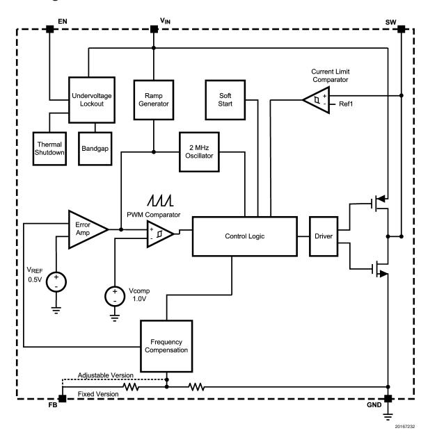
FIGURE 4. Simplified Functional Diagram
