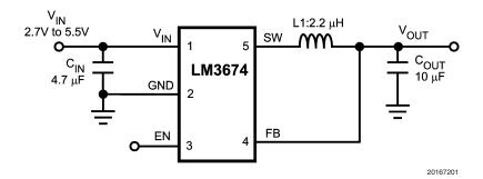
FIGURE 1. Typical Application Circuit
