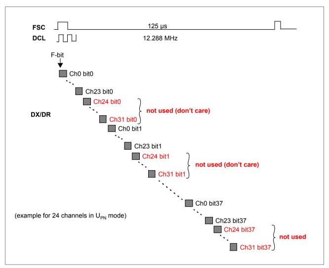
Figure 22 IOM-2000 Data Order (3 VIPs with 24 Channels)
