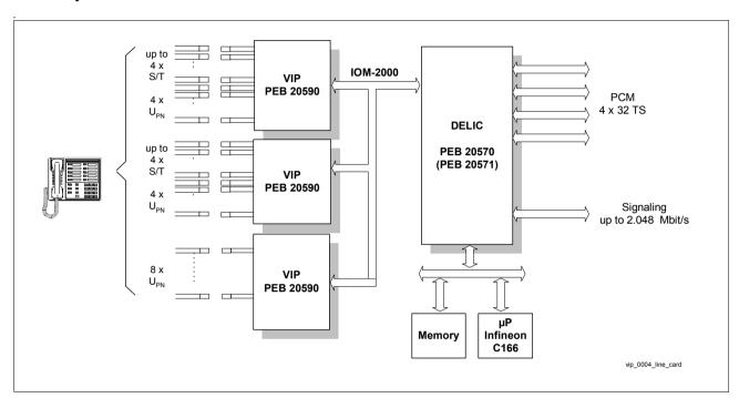
Figure 4 VIP in Mixed S/T and  $U_{PN}$  Line Cards (e.g. 8 S/T and 16  $U_{PN}$ )
