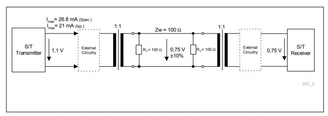
Figure 29 Overview of External Circuitry of the VIP in S/T Mode
