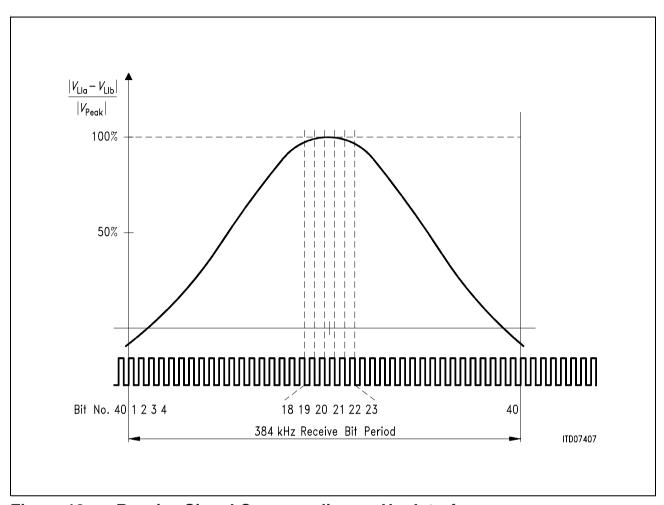
Figure 13 Receive Signal Oversampling on U<sub>PN</sub> Interface
