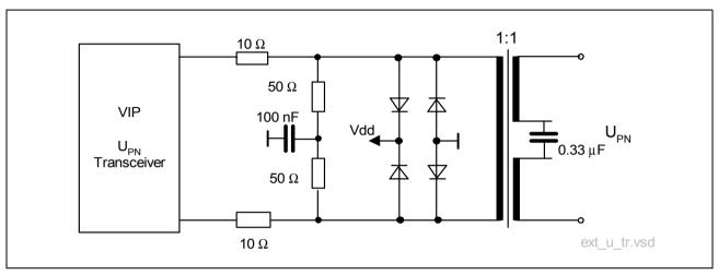
Figure 28 External Transceiver Circuitry of the VIP in U<sub>PN</sub> Mode
