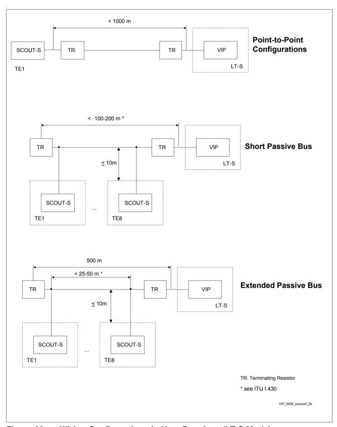
Figure 32 Wiring Configurations in User Premises (LT-S Mode)
