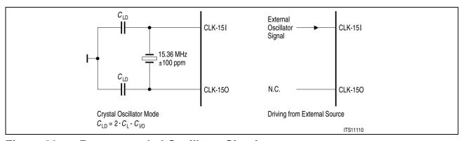
Figure 23 Recommended Oscillator Circuit
