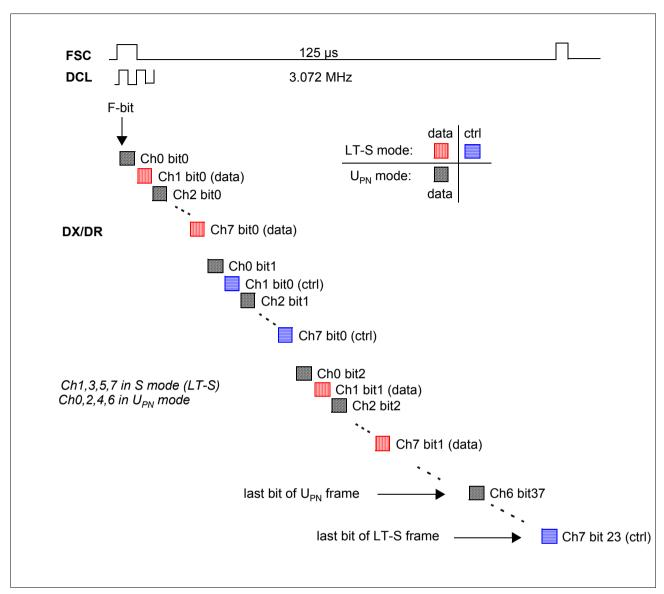
Figure 21 IOM-2000 Data Sequence (1 VIP with 8 Channels)
