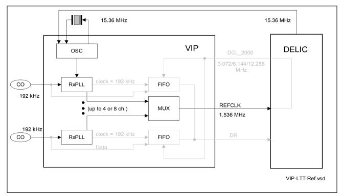
Figure 17 Clock Recovery in LT-T Mode
