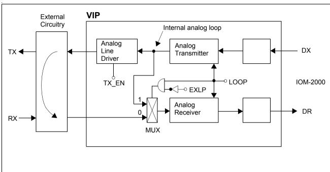
Figure 33 Internal and External Loop-Back Modes
