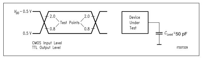
Figure 24 Input/Output Wave Form for AC Tests
