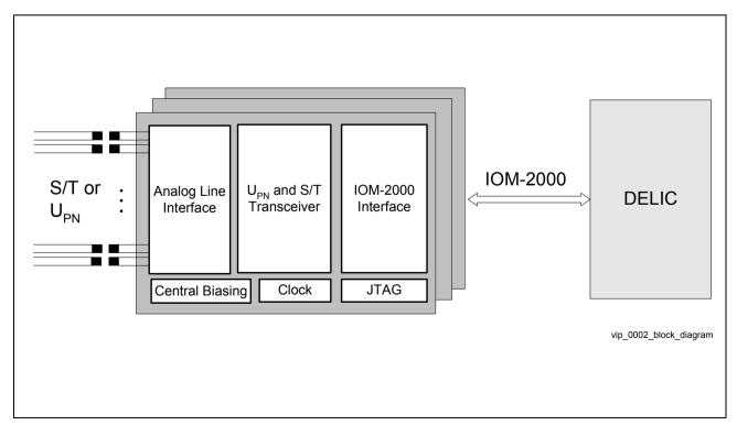
Figure 1 Top-Level Block Diagram of the VIP
