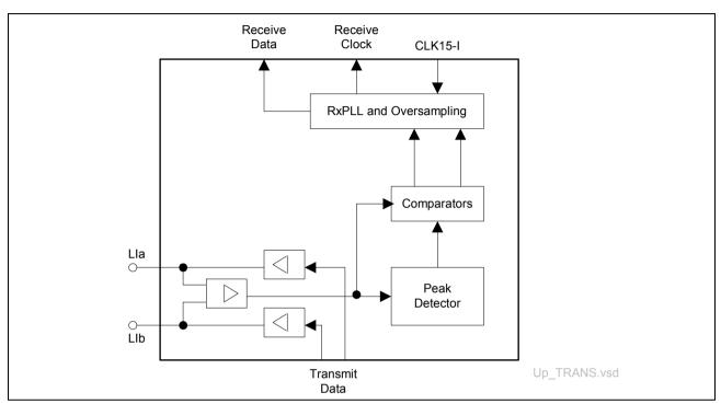
Figure 11 Transceiver Functional Blocks
