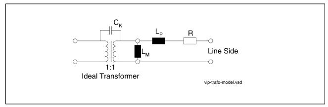
Figure 27 1:1 Transformer Model
