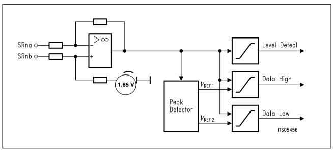
Figure 16 Receiver Functional Blocks
