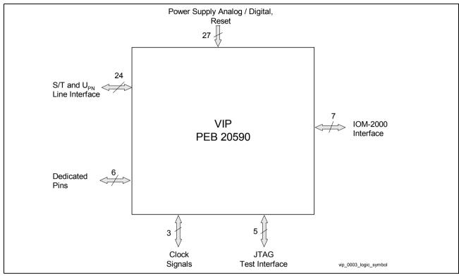
Figure 2 Logic Symbol PEB 20590 (72 of 80 Pins used)
