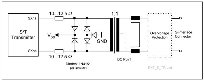
Figure 30 External S/T Transmitter Circuitry
