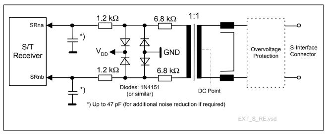
Figure 31 External S/T Receiver Circuitry
