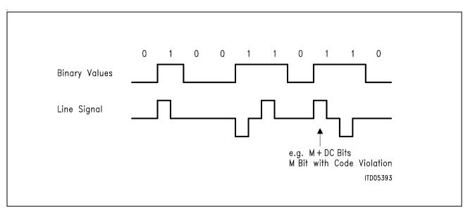
Figure 10 AMI Coding on the U<sub>PN</sub> Interface in VIP
