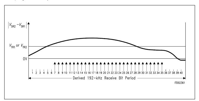
Figure 19 Receive Signal Oversampling in S/T Receiver
