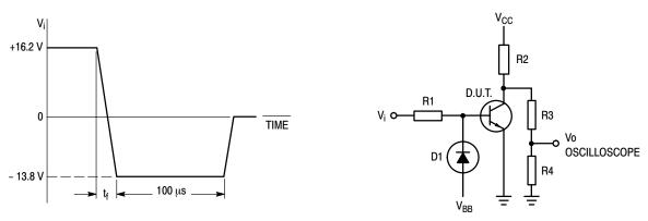
Figure 2. Input Waveform and Test Circuit for Determining Storage Time and Fall Time
