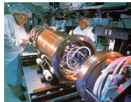
Telecommunications Undersea Cable Repeater
